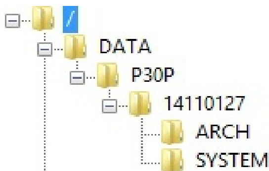
Fig. 20 The directory structure on the SD card.
